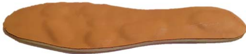
Fig. 2b. Image of foot inserts made with layered with polymeric foams at reflex points based on reflexology study
